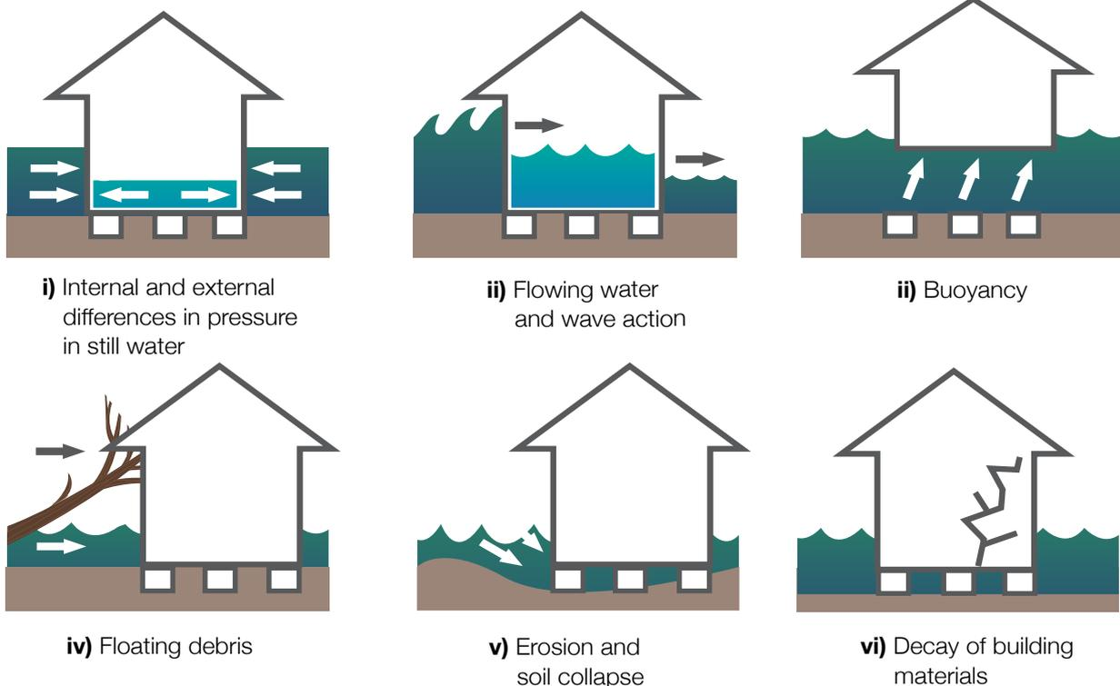
**Figure 1** Floods can result in structural damage of buildings in one of several ways.
